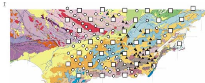
Figure 5: Planned locations of BBMT (open circles) and LMT (open squares) on the Betics. Existing BBMT sites also shown (solid triangles)
